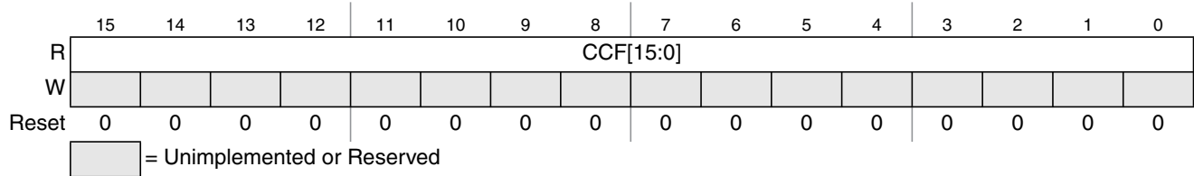
Figure 13-11. ATD Status Register 2 (ATDSTAT2)
